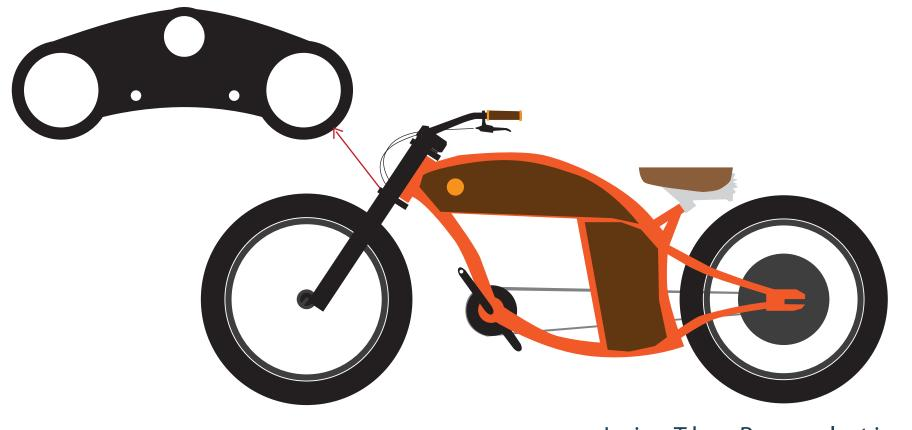
Place the light on the holes and screw the bolts
