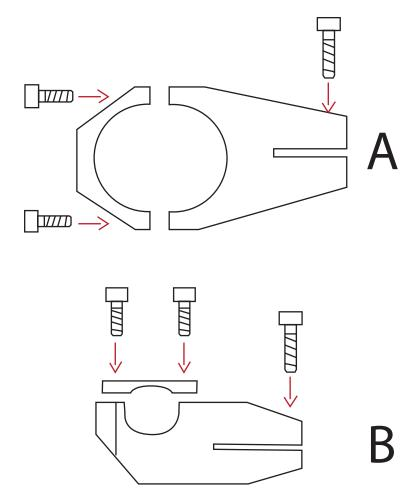
These are the position of the two pieces on the bike, this is a left view of the bike, the board carrier is always on the RIGHT side of the bike
