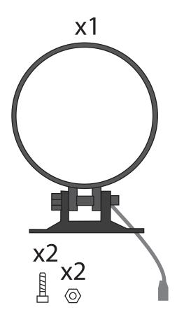
Locate the holes to place the front light. In the inferior plate of the fork there are 2two small holes to screw in the light
